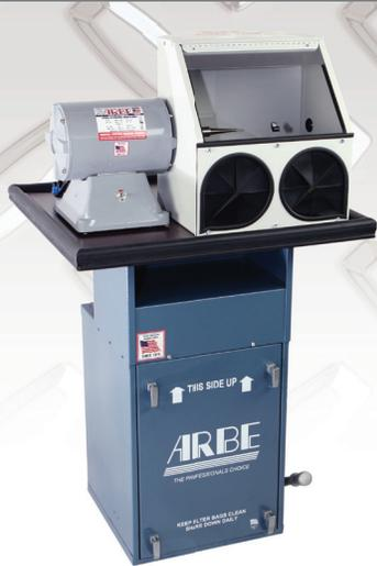
**Mini Floor Model Polishing System w/1/2 HP Dust Collector, 3/4 HP Single Spindle Polishing Motor and Enclosed Polishing Hood**
